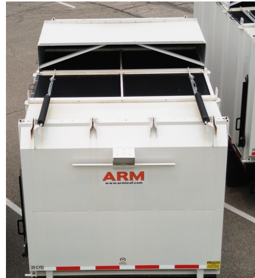
Hood air deflector shown above the hopper screening.
