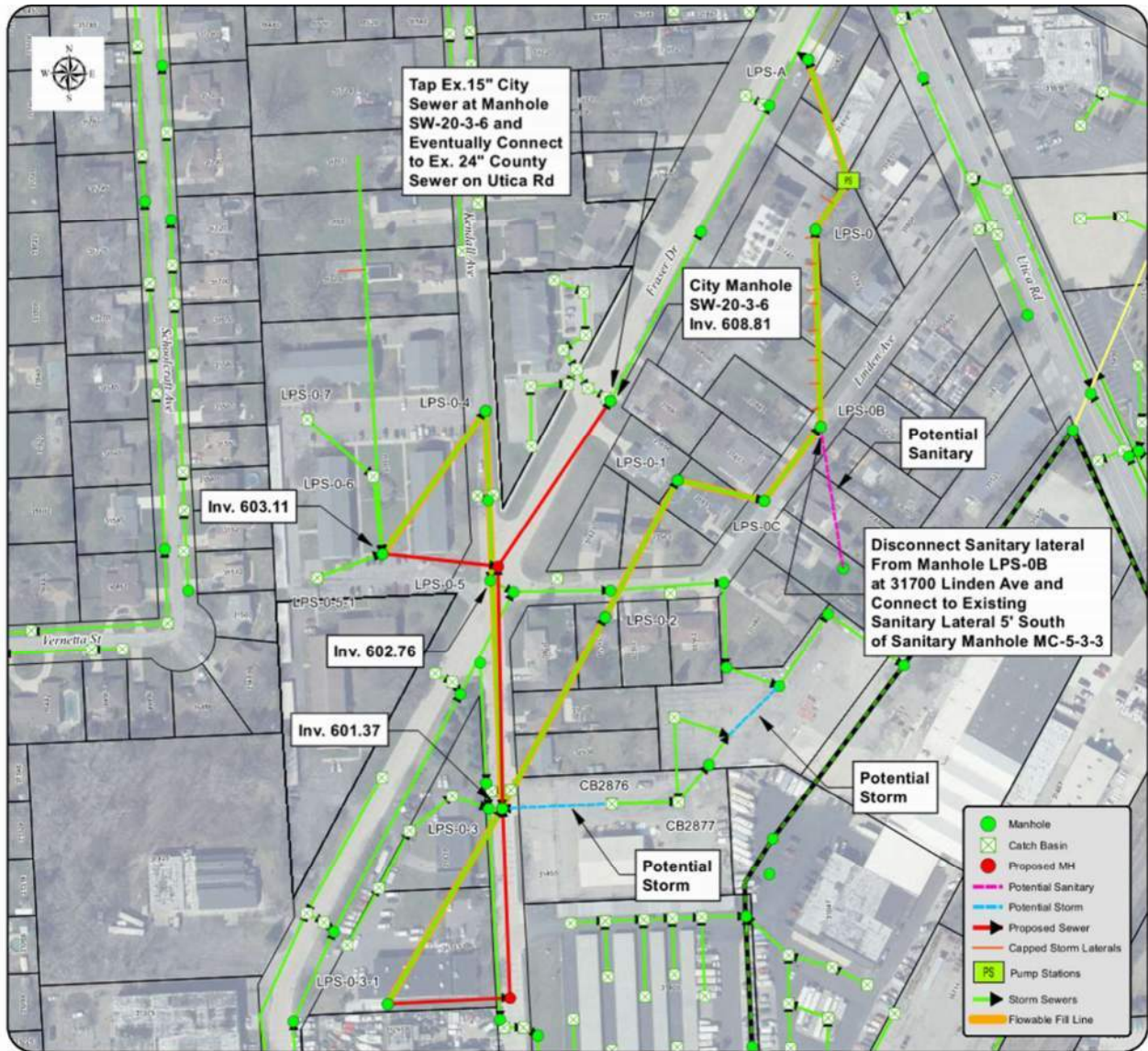
Figure 6: Option 1 - Re-route Flow to 15-inch City Sewer
