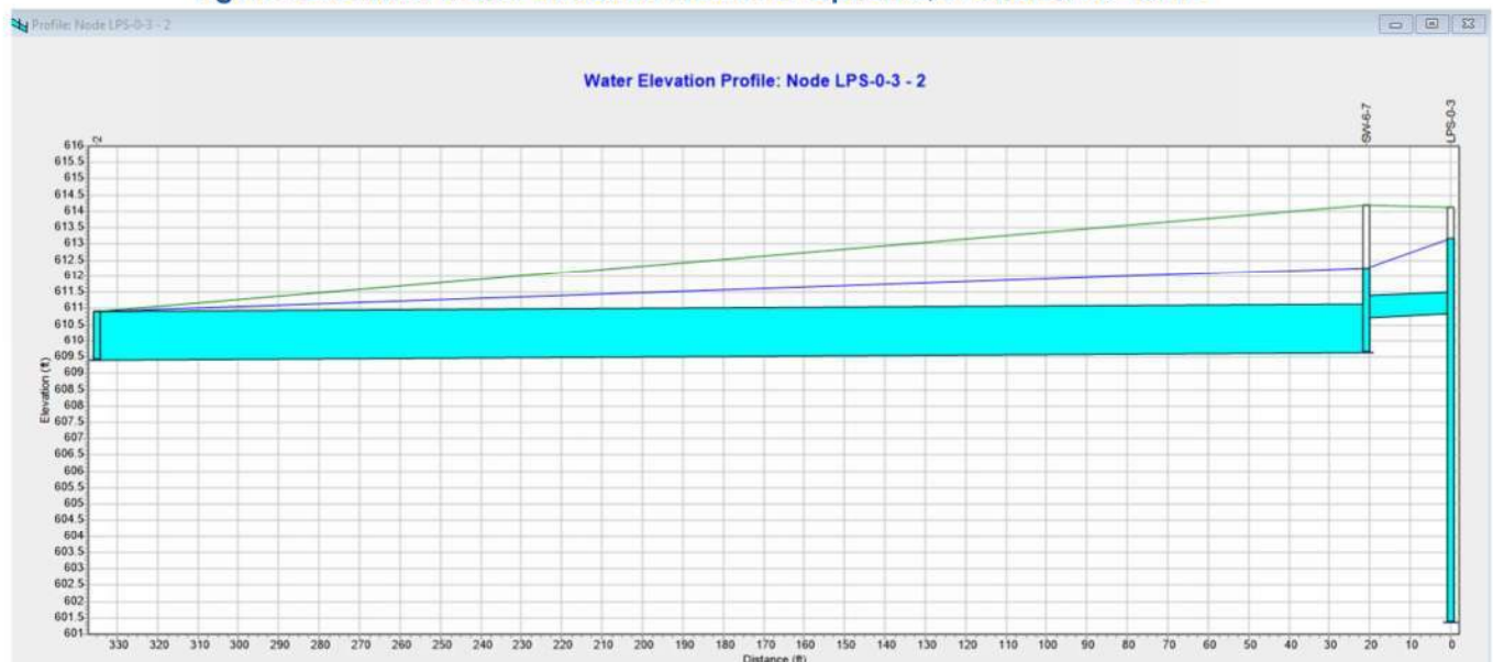
Figure 12: SWMM Water Elevation Profile for Option 3, Section 2 Re-route
