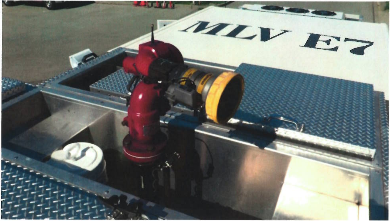
Example of remote deck gun/master stream device
